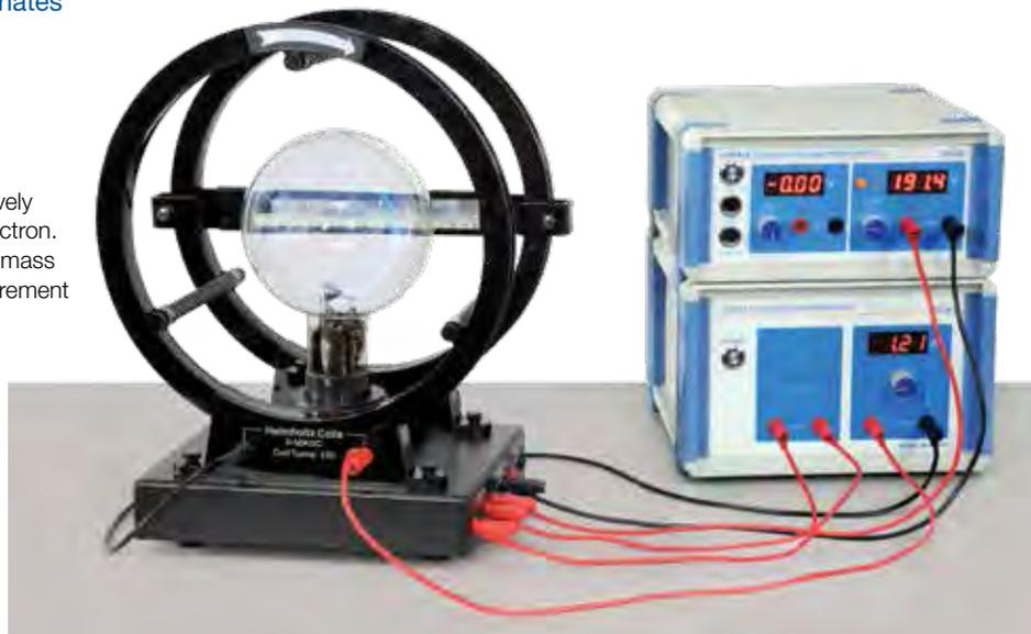
Complete Charge-to-Mass Ratio System includes the power supplies, which can also be used in other experiments (such as Franck-Hertz experiment, see page 305).
