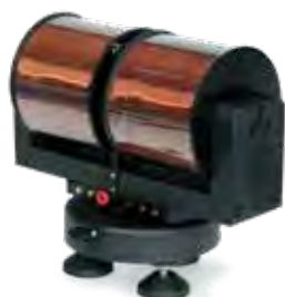
Electromagnet produces over one Tesla.
