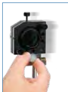
Lens and polarizer mount can be adjusted vertically and horizontally.
