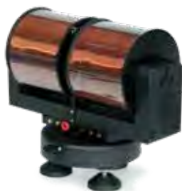
Electromagnet produces about one Tesla.
